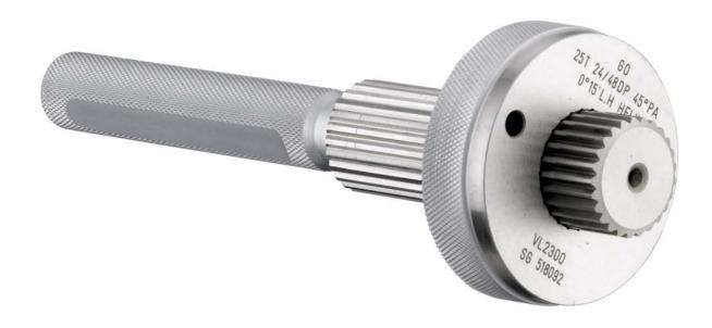
Taper tooth master plugs with fit and wear lines are used to monitor the wear of ring guages during component manufacture. The ring gauge is ground to fit the master plug for original and replacement ring gauges.
