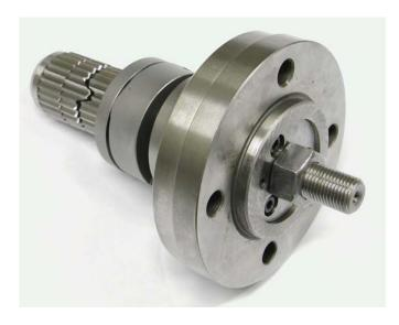
Machine face plate mounted mandrel.
