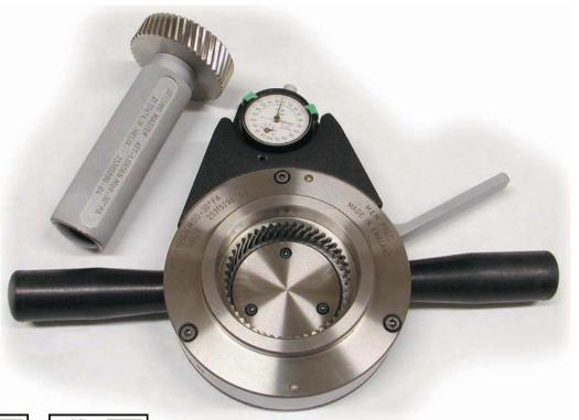
Can be supplied with analogue or digital indicators. Alternatively, a transducer port can be incorporated for SPC type analysis on PC.
